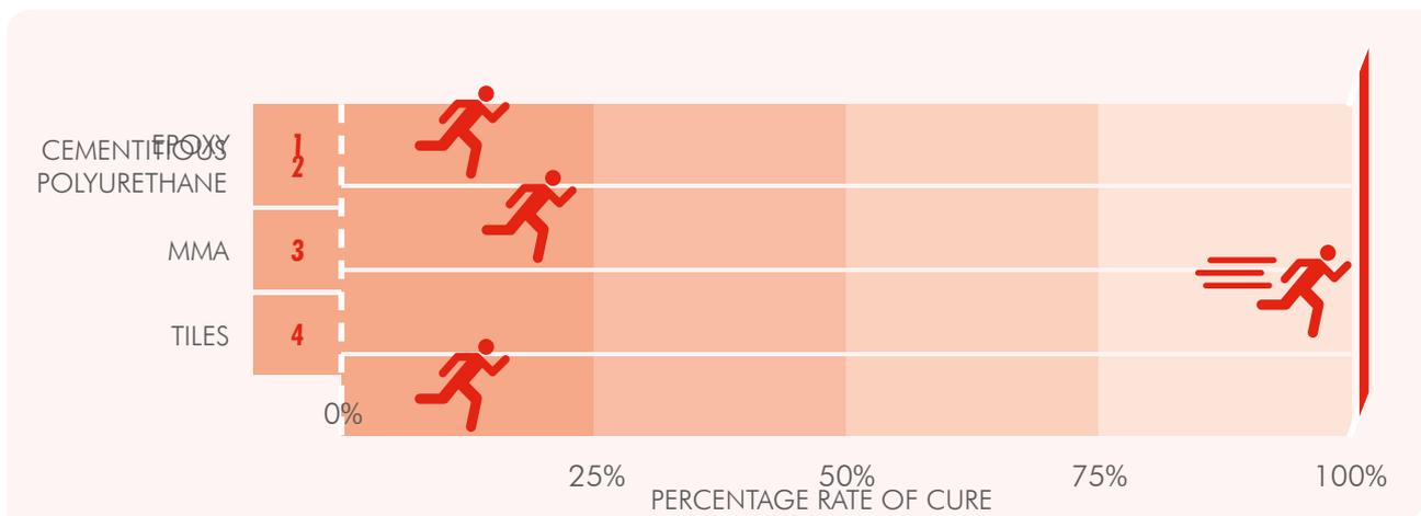
FIGURE 1: Hard Floor Coverings: Speed of Cure Comparison Diagram, Flowcrete Group Ltd, 2013. Controlled tests demonstrated that 100m<sup>2</sup> of MMA flooring took just 8 hours from preparation to full chemical cure and operational use compared to epoxy: 72 hours, Cementitious Polyurethane: 48 hours and Tiles: 72 hours.
